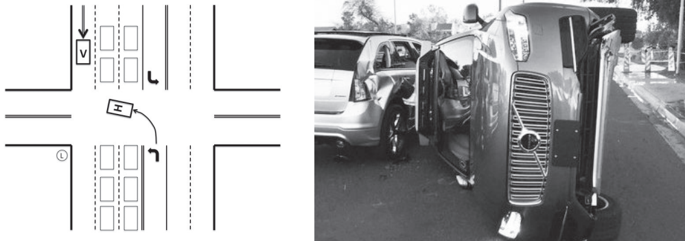
FIGURE 20: (left) Diagram of the situation leading up to the accident. The self-driving Volvo, marked V, is approaching an intersection, driving in the rightmost lane at thirty-eight miles per hour. Traffic in the other two lanes is stopped and the traffic light (L) is turning yellow. Invisible to the Volvo, a Honda (H) is making a left turn; (right) aftermath of the accident.
